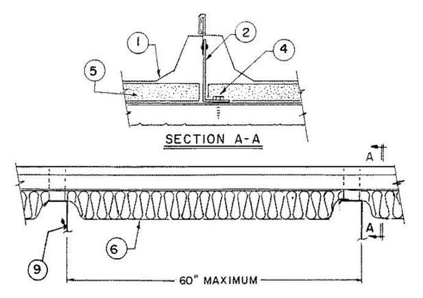
1. **Metal Roof Deck Panels\*** — For class 90-No. 24 MSG coated steel, for class 30-No. 26 MSG min. Coated steel, steel. Panels continuous over two or more spans. End laps to occur adjacent to purlins with panels overlapped 3 inch max. A line of sealant may be used at panel end and side laps.
